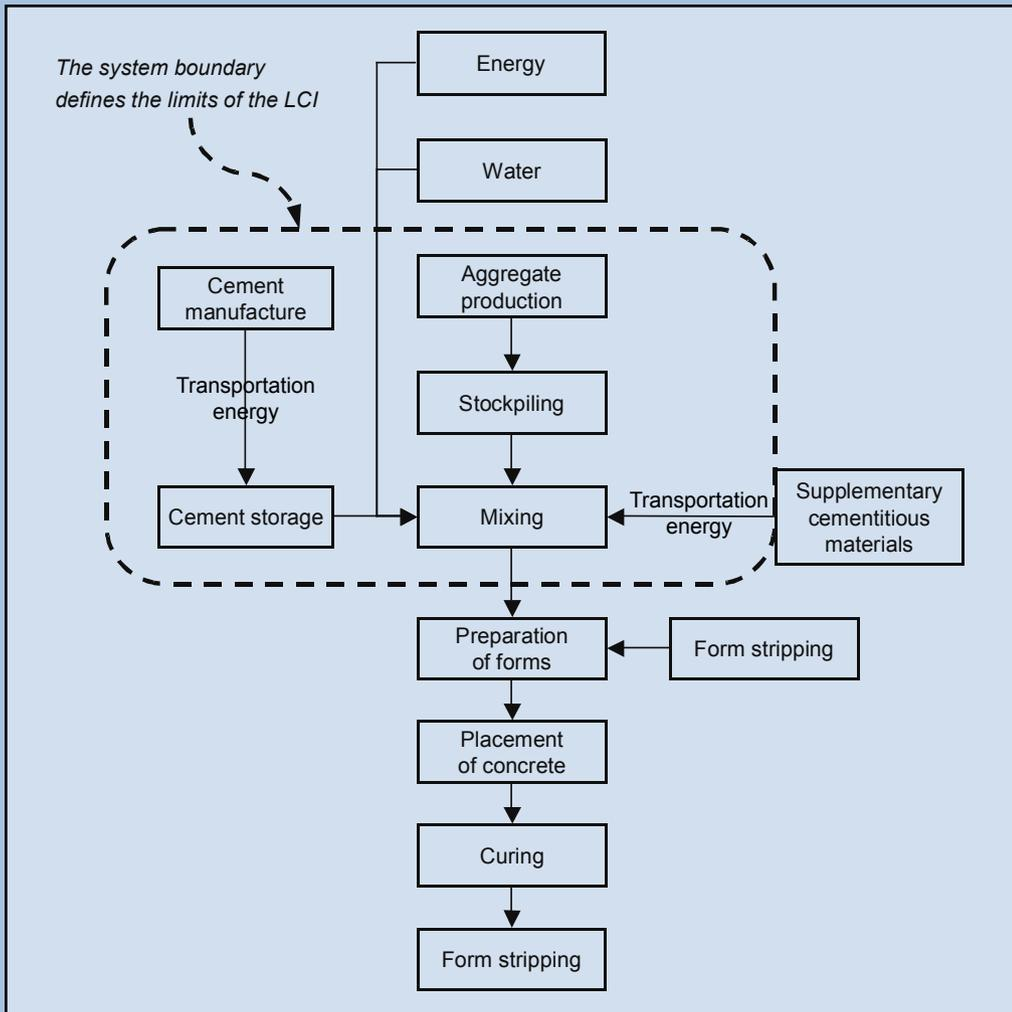
**Fig. 2.** Precast concrete system boundary
